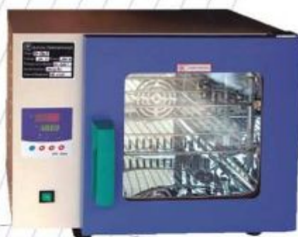
FO - 19053 1.9 Cu Ft 17x15x14" Ambient to 400 °F Forced Air Oven at $1,299
